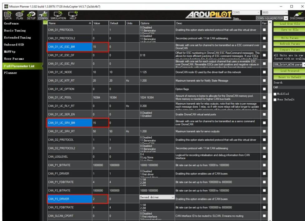
Note! Before using the flight controller to control the ESC, you need to make some simple settings:
